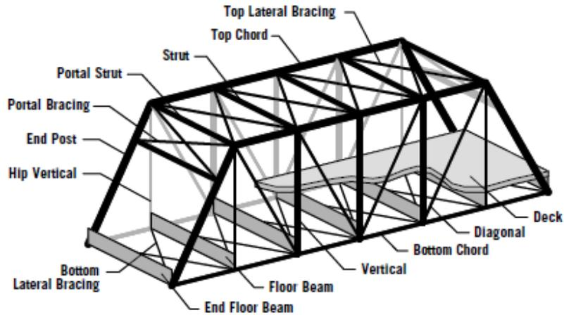
The three-dimensional bridge structure has two main load-carrying trusses. Each truss is composed of a top chord, a bottom chord, and several verticals and diagonals. The two trusses are connected together by a series of transverse members - struts, lateral bracing, and floor beams.
